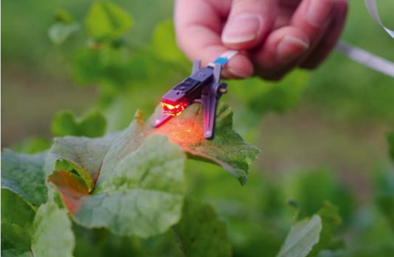
Prototype of a new sensor to make continuous photosynthesis measurements, developed by JII together with Michigan State University
